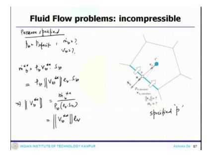
So, this case is a specified p. So, the pressure specified at the boundary which means my p b is specified and m dot b is not known. So, velocity b is also not known. So, one has to modify the equation of the mass flow rate correction mass flow rate would be rho b b V correction dot S b which will be rho b V b star star e V dot S b, which get you back the V b star star equals to m dot b star star divided by rho b e V S b which is V b star star and e V.
