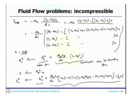
And, you can calculate the tau wall which would be minus mu b V c minus V b which is parallel d perpendicular minus mu b which can be written as V c minus V b minus sum V c minus V b dot n n and this is d perpendicular and you get all this component like u c minus u b minus u c minus u b n x V c minus V b n y plus w c minus w b n z multiplied with n x. So, this term would be common.
