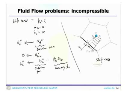
Now, similarly one can have slip wall. So, this is an example of slip wall and at slip wall what happens your p b is still unknown, mass flow rate is 0, force is 0. So, what one can modify that coefficients would be like this a c. So, this is only contribution come from interior faces and a F equals to b which 0 and b c is b minus b which is again interior faces and boundary faces.
