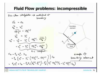
So, to do that let us start working on the boundary condition and this is a this is an example of an of boundary element. So, this is an example of an boundary element where you can see this is the boundary face and this is the cell center and this is the direction of that and this is the surface vector.
