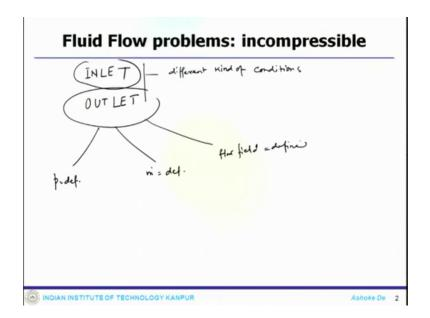
So, what we have done we have done the inlet boundary condition and under that umbrella different kind of conditions and now today, we are going to look at the outlet boundary condition. So, the outlet boundary condition could be also different type, different type in the sense could be static pressure defined, it could be mass flow rate defined, it could be a flow field defined so there are different ways one actually define the outlet boundary condition.
