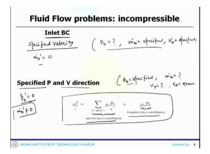
Now the second approach could be inlet boundary conditions. So, also in your domain there is a inlet condition, then the inlet boundary condition one can have let us say specified velocity. So, that could be one easy condition where specified velocity which means my p b is not known m dot b is some sort of a specified and v b is also specified.
