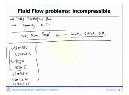
So, a apart from that there are few more which are also derive kind of conditions like also at the outlet one can have fully developed flow that could be one condition, then one can also have symmetry boundary condition. Now apart from that these are the some derived conditions.
