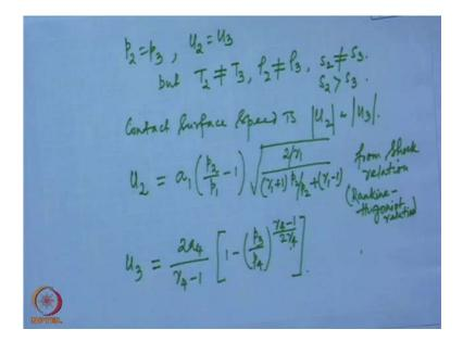
Now, on other side of this contact surface the temperature and density they can be different; however, the pressure and flow velocity they must be same that is on other side of the contact surface denoting by the appropriate symbol 2 and 3 we have p 2 equal to p 3 and u 2 equal to u 3; but, entropy as we have already seen that or other eventually entropy at region 2 is higher than region 3.
