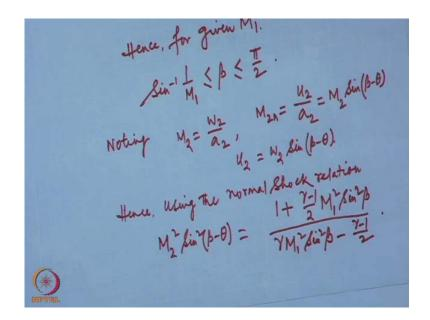
Hence, for a given upstream mach number M 1, the beta lies within the range of sin inverse one by M 1 less than beta or equal to beta less than equal to pi by two. For each wave angle beta, there is a corresponding deflecting angle theta. Now, to find the mach number downstream of the shock, we can obtain this by noting that M 2 equal to W 2 by a 2, M 2 n is u 2 by a 2 and u 2 is simply is M 2 sin beta minus theta and that is because u 2 equal to. (No audio between: 23:54-24:09).
