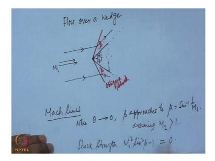
Now, this can easily be used to obtain the flow over a wedge. So, if we have a symmetric wedge and if we consider flow over a symmetric wedge, let us say flow over a wedge and of course, only supersonic flow. See, if the wedge is symmetric, ((no audio 48:43 to 49:13)) let us say that both are theta and the flow will be obtained by two oblique shocks at angle beta (No audio between: 49:33-49:58).
