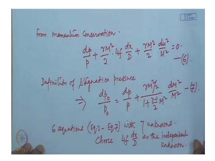
Similarly, from momentum conservation from momentum conservation, we get the same equation that we had in case of adiabatic flow with friction in a uniform area duct namely dp by p by gamma M square by 2 into 4f d x by D plus gamma M square by 2 du square by U square equal to 0, and from the definition of stagnation pressure this will be our equation six this gives us as before dp 0 by p 0 dp by p plus gamma M square by 2 divided by 1 plus gamma minus 1 by 2 M square into dM square by M square.
