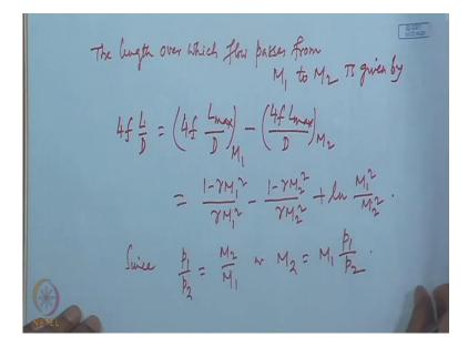
The length over which the length over which flow passes from M 1 to M 2 is given by 4 f L by D where L is this required length is 4 f sorry M 1 minus M 2, and using the relation that have been obtained for 4f L max by L max by D we get one minus gamma M one square by gamma M one square minus one minus gamma M two square by gamma M two square plus we have got M one square by M two square.
