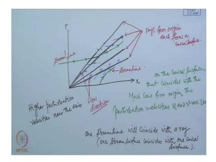
(No audio from 36:19 to 36:30) See, these are the x by r equal to constant line (Refer Slide Time: 36:32) (No audio from 36:42 to 36:57) and if we consider the complete axisymmetric body or complete axisymmetric case, so all these lines are generators and each of them form a conical surface. So, these are (No audio from 37:11 to 38:00), these are the rays from origin each forms a conical surface.
