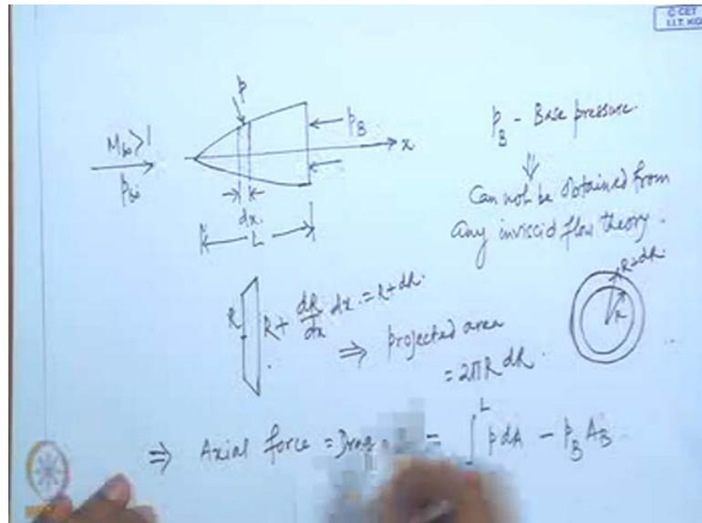
Now, let us come back to this pressure distribution once again (No audio from 35:33 to 36:13), we will consider a small section of length  $dx$  and the free stream as we have mentioned  $M$  infinity greater than the pressure here is  $p$  infinity. The pressure on the surface is  $p$  but, the back the pressure will of course, be different and will call that base pressure. Now, the pressure coefficient that we have obtained corresponds to this pressure.
