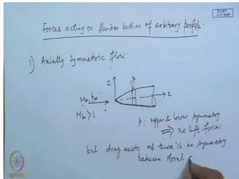
So, forces acting on slender bodies of arbitrary profile first, let us consider axially symmetric flow (No audio from 02:42 to 03:06), assume this body to be axially symmetric and the flow is along the axis. Now if we consider any small axial section over which the radius or you can say the cross-sectional area is increasing slightly, then we can see that the pressure that is acting on this strap where we have  $m$  infinity is a free stream speed when the free stream pressure is  $p$  infinity.
