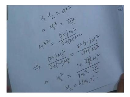
So, what we can see from here that when the flow is subsonic at station 1, the flow is likely to be supersonic at station 2. Similarly, if the flow is supersonic at station 1 it will be subsonic at station 2. However, there is nothing in this relation that excludes this one of these possibilities. However, as I mentioned that based on physical ground that if there
