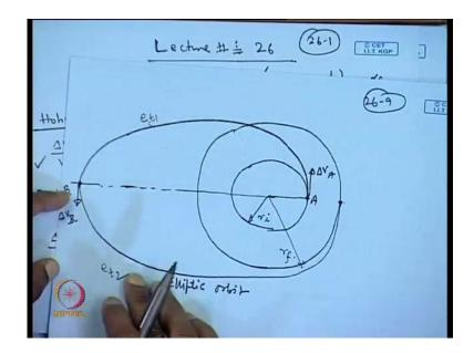
So, in the bi elliptic transfer what we have done, this is the initial orbit given, whose radius is r i, and this is the final orbit given whose is r f. So, bi elliptic transfer, we transfer from point A to point B, and here the impulse delta v A was given and then again the impulse here delta v B was given, and then it is transfer to this point, and in an elliptic orbit, this is the elliptic orbit. So, we can write this as the eccentricity of this orbit
