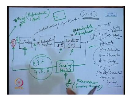
Now, let us say, we have a satellite, which is shown by this block diagram. Often, we indicate it by P, to indicate this is a plant. So, to maneuver the satellite in the orbit, you need certain amount of movement along the different axis. Without that it cannot be maneuvered. So, those movements can be passive movement, or it can be the active movement. So, what is the passive movement, active movement, we will come next to, in this discussion.
