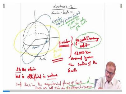
So, what I have shown here, this is say our earth and around the earth, we need to put satellite, so satellite can be put in various orbits around the earth, so if we have an orbit which is in the equatorial plane of the earth, so this is in the equatorial plane of the earth and if it has a period of 24 hours, 24 hours period then and the orbit is circular, so such arbitrary call as the geo stationary orbit.
