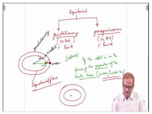
So, equatorial orbit we are dividing into 2 parts; one is geostationary, another one is geosynchronous, 24 hours period and also here 24 hours period, now it is; this is not the only orbit possible, if I have the earth equator here, so I can have satellite at the altitude of even 300 km, so from distance from the surface of the earth to this place, this is 300 km but then we will not call this as either geostationary or geosynchronous.
