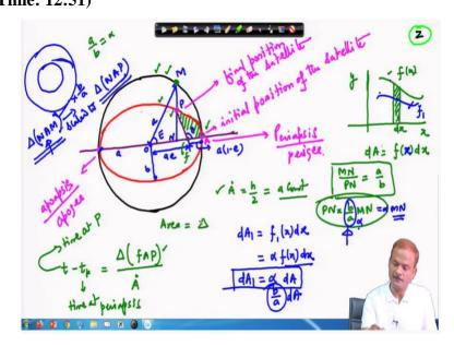
So, what we are going to do we are going to find out the Kepler's equation using the graphical method. So, this represents a and b. I am not showing here b you can show here in this place and this is b so this is your half of the semi-major axis from this point to this point this is a this distance is as usual a (1- e) in the case of ellipse and distance from this point to this point and this is ae.
