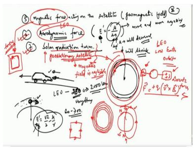
So, this term we are calling as the indirect oblation perturbation term, then we have other terms like the magnetic forces acting on the satellite, this is because of the earth's magnetic field, geo magnetic field acting on the satellite, this is the geomagnetic field. Then the aerodynamic forces; aerodynamic force, solar radiation term, okay. So, aerodynamic force this especially needs mention as you know for the ellipse, we write it like this as specific energy.
