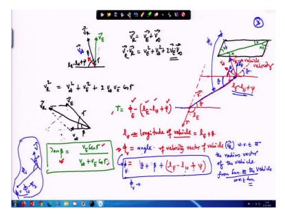
Then we go to the vehicle so it is shown that the  $V_{\infty}$  it is in this direction and  $V_{\infty}$  is shown like this.  $V_{\infty}$  is shown like this and then the  $V_E$  were shown by proper colour. This is the V Earth and  $V_R$  resultant is shown in black. So the resultant is  $V_R$ , this angle we have written as  $\beta$  and from here to here this we write as  $\gamma$  moreover an angle with the horizontal angle as shown here is  $l_E - l_H + \psi$ .
