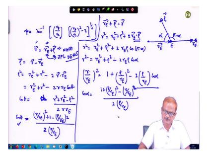
Now we have start working with the angles. So already last time we have derived this relationship  $\Psi$  is equal to tan inverse V<sub>P</sub> by V<sub>C</sub> times square - 2 whole power 1 by 2 this is the relation last time we have got. Also, we can observe from the previous figure that this  $\vec{r}$  this vector will be nothing but r will be  $r_E + \rho$  where  $\rho$  is the vector till the vehicle. As shown here this is a  $\vec{\rho}$  this is your  $\vec{\rho}$ .
