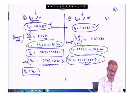
So in the next trial I made it  $\theta_A$  is equal to 15°. So the corresponding value for the  $e_t$  then turns out to be because I programmed it. So it was easy for me to do this problem. And  $r_A V_A^2$  this is for the transfer orbit remember. This turns out to be 2.1505. Semi major axis this turns out to be; so you can see that this eccentricity has been reduced. The reduction of the eccentricity earlier it was 1.5 something 1.59.
