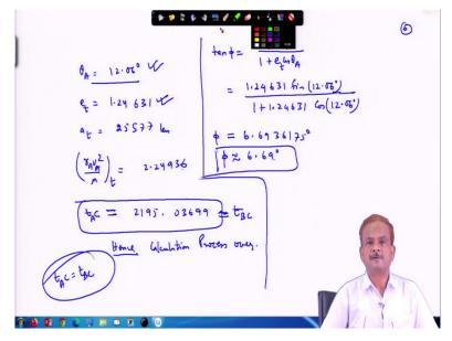
So, in the next trial we choose  $\theta_A$  is equal to 12.06°. So corresponding e t will be turnout 21.254631 A transfer orbit 25577 and  $r_A V_A^2$  divided by  $\mu$  in the transfer orbit this turns out to be route to reach 2.24936 and t<sub>AC</sub> the transfer time 2195.03699. So, it is very close to the t<sub>BC</sub>.
