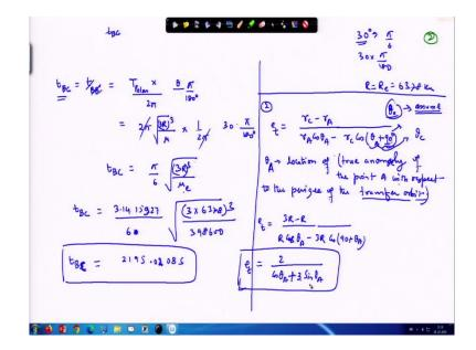
So, going from time from B to B' or the same thing last time we have written as BC. This time will be the time period in the orbit. This orbit is circular orbit so how much time it will take to go from this place to this place. So, t BC' or BC let us make it t only to be consistent with the last time. So,  $t_{BC}$  so the time period in the polar orbit and this as to be divided by the corresponding 2 $\Pi$  and multiplied by corresponding the angle to which the satellite is going from B to C.
