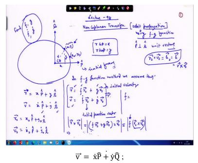
So I have written here the orbit propagation you see using the f - g function. So what does this mean? Let us look into this figure which shows here as an ellipse ok. However, it may be anything. This is the co-ordinate XY this is r and this angle is e  $\cos \theta$ . So, r  $\cos \theta$  is equal to X and then r  $\sin \theta$  is equal to Y.  $\hat{P}$  and  $\hat{Q}$  these are the unit vectors along the; basically, in the Plane of the orbit the co-ordinate axis.
