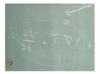
Okay so in Lagrangian frame of reference you would simply look at a rate of time rate of change of species mass fraction Yi as far as this is concerned all right, so this is actually together then called inertial term okay. (Refer Slide Time: 43:06)
