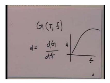
So, there is a quantity called Gibb's free energy, which is often denoted by G. This Gibb's free energy is a function of temperature and is a function of the force or the pressure. So, here is the force. So, you can measure the Gibb's free energy and the value of the Gibb's free energy depends on, how much temperature, what is the temperature of the system and what is the force you apply. So, this, in this case, the case of unzipping,
