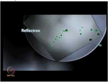
The Reflectron compensates for minor velocity differences improving the resolving power of the 6510.
