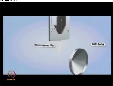
The HPLC chip loading mechanism precisely and optimally positions the electrospray tip orthogonal to the MS inlet for maximum sensitivity and robustness, day-in, day-out.
