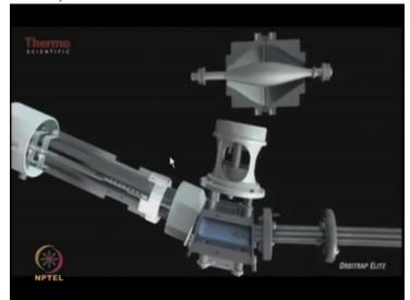
Expert: The c-trap does cooling the ion and makes it into the packet of ion, so that the packet of ion injected
