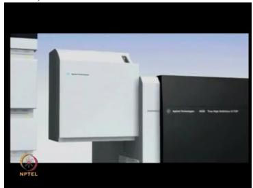
... the Agilent 1200 series HPLC chip/MS interface; the chip cube. The chip cube includes an electrospray ion source with optics for spray visualization, HPLC chip loading and ejection mechanism, nano LC connections and micro-valve switching.
