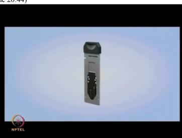
The compact architecture of the Agilent HPLC chip reduces peak dispersion and combines all steps from sample loading through compound ionization for seamless operation.
