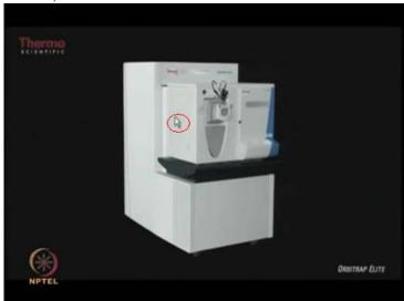
Expert: the mass spectrometer which is sitting in front as a linear trap, Velos, LTQ Orbitrap Velos...
