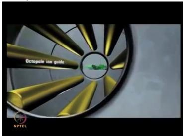
Another Octopole ion guide keeps the ions together while allowing excess collision gas...
