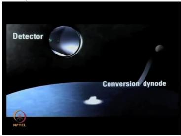
...Conversion dynode operates at 10000 volts to improve sensitivity; because the conversion dynode is off the main axis of the ion path...
