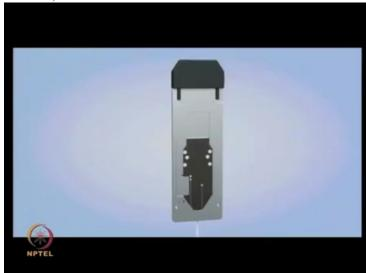
With the Agilent 1200 series nano LC system including microwell plate auto sampler and loading pump connected directly to the chip cube, an HPLC chip is loaded and ...
