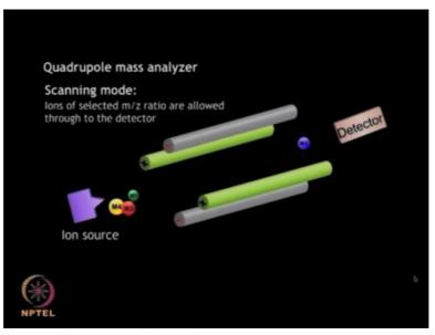
In the scanning mode, the quadrupole analyzer selects ions of specific m/z value as said by the user. A range can also be (()) (27:10) in which case only those specific ions which satisfy the criteria will move towards the detector and rest can be filtered out.
