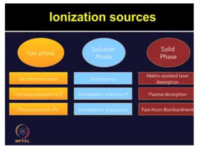
With the gas phase electron ionization, chemical ionization and photoionization; these are the more commonly used ionization sources. With solution phase electrospray, atmospheric pressure and atmospheric pressure CI; these are the more commonly used ionization sources. With solid phase MALDI or Matrix – Assisted Laser Desorption Ionization, plasma desorption are the more commonly used solid phase ionization sources.
