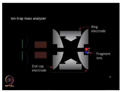
Now let us discuss the next mass analyzer, ion - trap. An ion - trap make use of a combination of electric and magnetic fields and captures ion in a region of a vacuum system or tube. Ion - trap traps the ion using electric field and measures the mass by selectively ejecting them to a detector.
