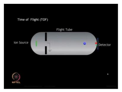
The Time of Flight accelerates charged ions generated by the ionization source MALDI along a long tube known as the flight tube or TOF. Ions are accelerated at different velocities depending on their mass to charge ratios. Ions of lower masses are accelerated to higher velocities and reach to the detector first. The Time of Flight under such circumstances is inversely proportional to the square root of molecular mass of the ion. The TOF analyzer has several applications in the proteomics.
