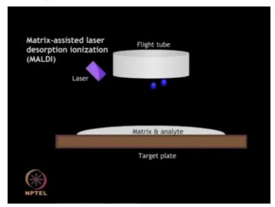
Let us discuss the 2 most commonly used soft ionization techniques MALDI and ESI in more detail. In MALDI, the analyte of interest is mixed with an aromatic matrix compound such as
