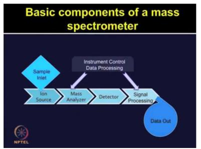
Sample inlet: It transfers a sample into the ionization source. The ion source or ionization source: It converts neutral sample molecules into the gas phase ions. Mass analyzers: It seperates and analyses mass of the ionic species. There are various type of mass analyzers available which we will discuss in more detail during the subsequent part of the lecture. Now I need to maintain the vacuum condition.
