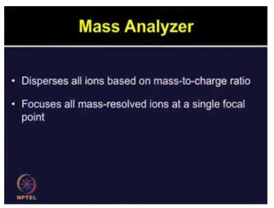
First of all, it disperses all the ions based on their mass to charge or m/z ratio. Second, it focuses all the mass – resolved ions at a major single focal point. So therefore, all the ions enter in the mass spectrometer, it can maximize their transmission.
