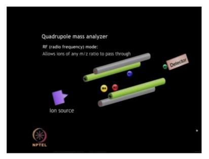
Quadrupole: The quadrupole mass analyzer use oscillating electric fields to selectively stabilize or destabilize the parts of ion passing through a radio frequency quadrupole field. The quadrupole mass analyzer can be operated in either radio frequency or scanning mode. In RF mode or radio frequency, ions of all m/z are allowed to pass through which are then detected by a detector.
