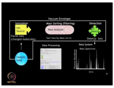
Mass spectrometer is an instrument that produces charged molecular species in vacuum, separates them by means of electric and magnetic fields and measures the mass to charge ratio and relative abundance of the ions that produced. It is being increasingly used for detection and analysis of proteins from the complex samples. The various components which are involved in the Mass Spectrometry experiment are shown here.
