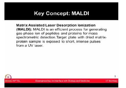
It is one of the efficient process for generating gas phase ions of peptides and proteins for the mass spectrometry detection. In this, there is a target plate which has a dry matrix and the protein sample which is exposed to a short, intense pulse of a laser light.
