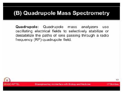
So this mass analyzers, they use oscillating electric fields to selectively stabilize or destabilize the path of ions which is moving inside these quadrupoles and then they are passing through the radio frequency of these quadrupole field. So this is one of the, again, one of the popular configuration.
