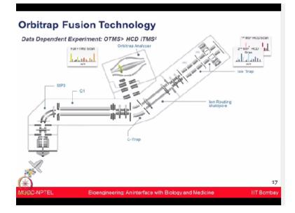
So in this manner, one of the latest technology which has come forward is orbitrap fusion technology where we have quadrupoles, ion trap and orbitraps and both ion trap and orbitrap have their own detectors as well. So now, you know, this kind of tribrid technology not only provides the highest resolution but also provides, you know, multiple capability to do different type of fragmentation, different ways of analysis and it opens up many type of applications by using this kind of technology.
