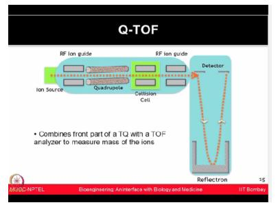
It utilizes 2 different mass analyzers based on, the first one is a quadrupole property and second one is the time of flight. So not only you are resolving them in the electric field but also separating them based on the Time of Flight tube, looking at the mass to charge ratio, how much time they take to separate them.
