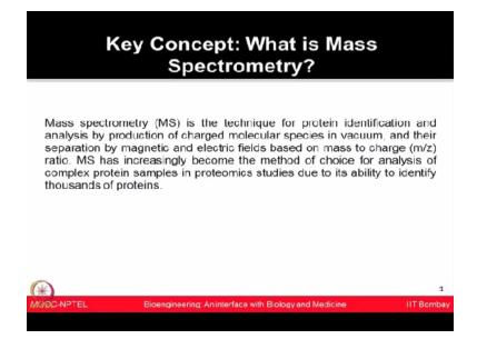
So what is mass spectrometry? It is a technique for protein identification and analysis by producing the charge molecular species in vacuum and then their separation by magnetic and electric field based on the mass to charge ratio. This technology has become increasingly in use in the proteomics field and now has become a method of chaise for analyzing the complex protein samples for proteomics studies.
