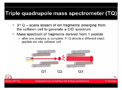
And then in the third quadrupole, you are scanning the stream of these ion fragments which is emerging from the collision cell which generates the CID spectrum. So therefore, by utilizing these properties of mass analyzers, different type of mass spectrometry configurations have come forward. Now I have shown you this mass spec which is Q-TOF or quadrupole Time of Flight.
