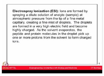
Let us now talk about another ionization method which is electrospray ionization or ESI. In ESI, the ions are formed by spraying a dilute solution of analyte at the atmospheric pressure from the tip of a fine metal capillary and that creates a fine mist of droplets. These droplets, they are formed in very high electric field and becomes highly charged.
