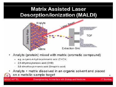
And that is going to generate these ionized forms of these peptides which could be further analyzed in the mass analyzers. So here in this image, it is shown that analyte or the protein of interest is mixed with the matrix which could be some aromatic compound, it could be different type of matrix could be used like alpha-cyano-4-hydroxycinnamic acid or it can be 2,5 dihydroxybenzoic acid or DHB. It could be Sinapinic acid.
