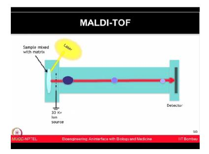
You can see this in this diagram that, you know, laser is bombarded. Now these ions are based on the mass to charge ratio, they are flying inside the Time of Flight tube and reaching to the detector.
