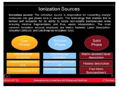
The soft ionization is known for its ability to ionize non-volatile biomolecules while ensuring the minimal fragmentation and therefore, one could easily interpret the data. The most commonly used ionization methods include electrospray ionization or ESI or matrix assisted laser desorption ionization method which is MALDI. Let us first talk about MALDI or matrix assisted laser desorption ionization method.
