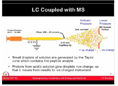
So this is small droplets from a solution forms are generated that is known as a Taylor cone which contains the peptide analytes and now the protons from the acidic solution, they provide droplets a positive charge so that now it can move to the negatively charged instrument and both by using the differential pressure and the charge, you are trying to move all these ions which are coming from the peptides towards the mass analyzer.
