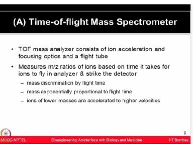
The TOF mass analyzers, it consists of the ion acceleration and the focusing optics inside the flight tube. It measures the mass to charge ratio of ions based on how much time it takes for the ions to fly inside the analyzer and how much time it takes to strike to the detector. So you are using mass discrimination based on the flight time and the mass is exponentially proportional to the flight time. So ions of lower masses are accelerated to the higher velocities here.
