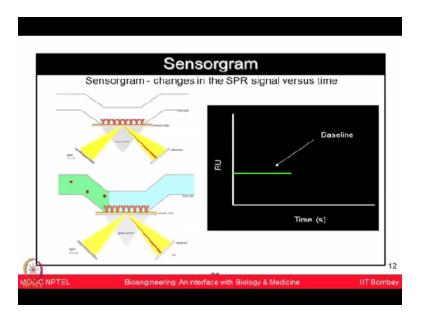
So for example, as you can see in the plot, on the x-axis, we have the time scale. On the y-axis, we have response units and then we are looking at from the baseline initially when there is no interaction happening, the stable baseline is there. And as soon as the 2 molecules start interacting, from those molecules you can see now the association rate can be seen in the green curve if you are seeing. Now the binding can be seen.
