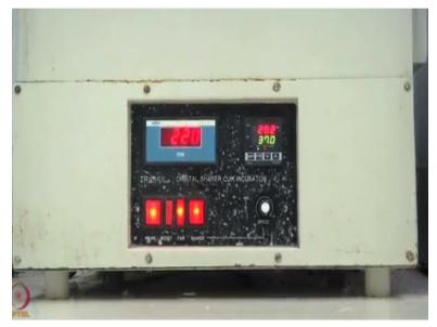
So, this is the shaking incubator in which I will keep this tube for overnight incubation. So, you can see the temperature set is 37 which are ideal for the bacterial growth.
