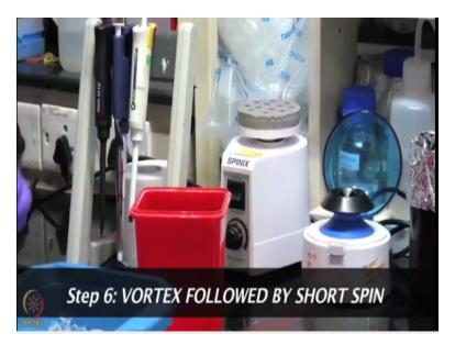
So, this is the ligation buffer, I will give it a small vortex, I will add this to the ligation makes now, the last thing to be added is the ligase enzyme again, we are using a small pipette because we require very little quantity of the enzyme, I will give it a short vortex again to the enzyme, now our ligation mix is ready, we will vortex it a little, followed by a short spin.
