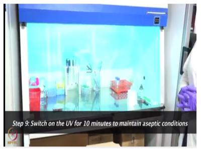
So, before we start with the experiment, first we switch on the UV for 10 minutes, this step ensures that inside the conditions are extremely sterile, this step ensures that inside the laminar hood conditions are extremely sterile under good for a work. So, after this we will switch off the UV and we switch on the fan and the light button.
