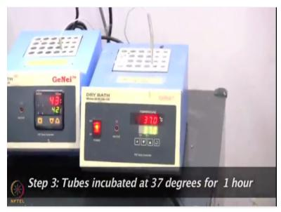
So, the incubation will be done for 1 hour, so after restriction, digestion has been performed. (Refer Slide Time: 07:46)
