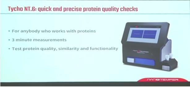
So what's the basic principle of this machine is that it can work with any kind of protein, whether its antibody or whether it's a normal protein, membrane protein, receptor protein, any kind of protein and it give a 3 minute measurement, so within 3 minutes you are actually checking your quality and the purity of the protein, so it's a label free measurement, like here one of the partner is labeled,
