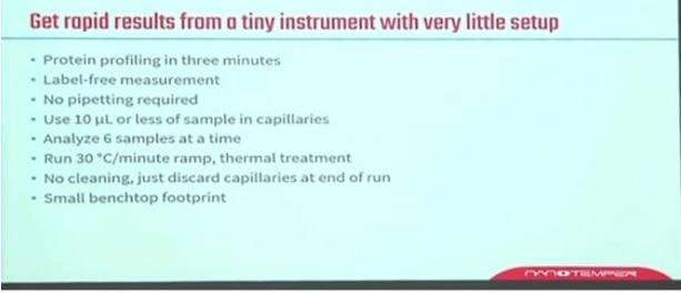
we are not labeling here, it's the intrinsic protein fluorescence that we are checking which will give you a label free, what you call inflection temperature which is very equivalent to the melting temperature.
