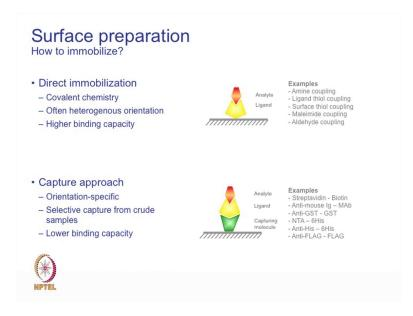
Immobilization is done by direct method as we just discussed and that immobilization can be by covalent chemistry and there will be high binding capacity. And, the ways the very examples of a direct immobilization are amine coupling, thiol coupling, aldehyde coupling, maleimide coupling are the methods that are available.
