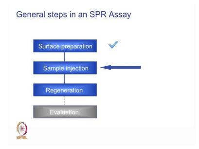
The various steps that are involved in a Biacore assay are surface preparation, sample injection, regeneration and evaluation. So, we will start with the surface preparation.
