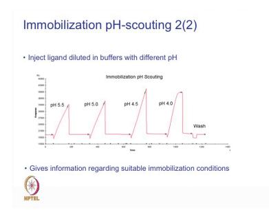
In this process if we sometimes are not aware of a pI because the molecule is a new molecule and it is just recombinantly expressed and we do not know the molecular isoelectric point in that case we will go for an immobilization pH-scouting in which we will dissolve the protein at different pH and then we tend to pass on the surface of the chip and see what is the responses that are coming up from the molecule.
