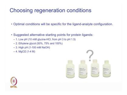
And, some of the very natural or regular usage of regeneration conditions are low pH, ethylene glycol, high pH and magnesium chloride. So, once we identify the proper regeneration solution it is very important for us to identify once we use this regeneration condition are we getting our reference surface on our active surface back after injecting this reference?
