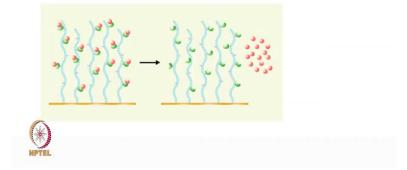
Regeneration as I just said removes the bound analyte completely from the surface. The activity of the surface must remain unaffected after regeneration and an efficient regeneration is crucial for a high quality data. And, regeneration conditions we need to test the regeneration surface, we can do a regeneration scouting before start of an assay or a develop and assay and then identify the right or the appropriate regeneration conditions.
