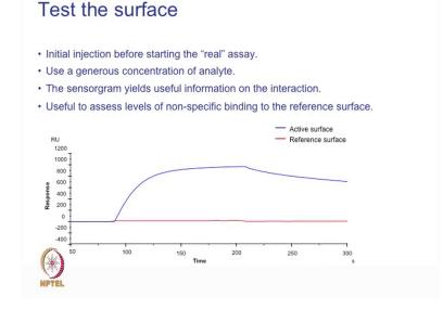
Then it is a very good way to start by injecting a small amount of your sample to see what is the binding responses that you are getting and to what time you should continue your binding and went to dissociate and all that. That process is called test of a surface you can just test the surface to understand the interaction and also understand the regeneration condition and level of non-specific binding that is coming up from these interactions.
