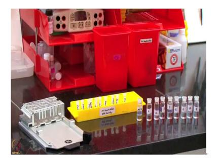
We will now proceed to insert these tubes including the sample the startup 50 percent DMSO and the solvent correction solution into the appropriate racks and then into the system to perform the protein small molecule screening assay.
