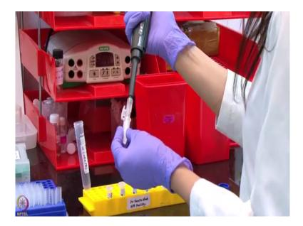
We will prepare this concentration series in twofold dilution using running buffer starting from 20 micromolar; which means, we will make 200 microliter of 20 micromolar protein with 200 microliter of running buffer to get the 10 micromolar concentration.
