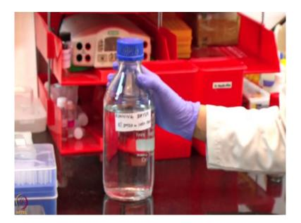
In this study, we will again be using 5 percent DMSO in 1.05X PBS as the running buffer which will also be used for the initial startup cycle.
