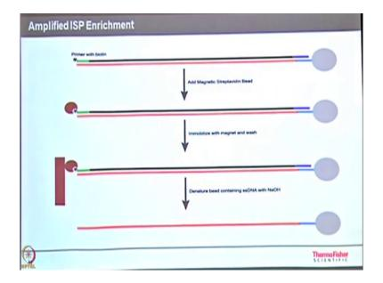
And then we just go through. So, this is primarily your ion sphere this will have these molecules all over because we clonally amplified. So, you use streptavidin coated beads and this streptavidin streptavidin coated beads are magnetic. So, with the help of a magnet all these are fished out and then you have only the beads which are amp which have amplified which are finally, to be loaded on the chip.
