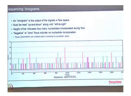
So, this ionogram is again being read by the sequencer, this has to be read from left to right and for the number of bases. So, whether you get a signal or not that will define the sequence of the dNTPs, the intensity of the signal will define how many of those dNTP how many of those As or Ts were in a row.
