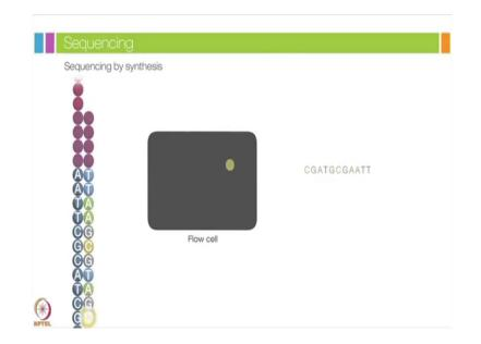
Only one is incorporated based on the sequence of the template. After the addition of each nucleotide the clusters are excited by a light source and a characteristic fluorescent signal is emitted, this proprietary process is called sequencing by synthesis.
