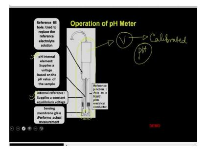
So, in a pH meter as I said you know you have a pH electrode and this pH electrode is going to be dipped into the solution where you are actually interested to measure the pH, but before doing that because the this pH electrode only knows that what is the voltage difference between the internal electrode versus the reference electrode. So, this V has to be calibrated with the help of the different pH solutions.
