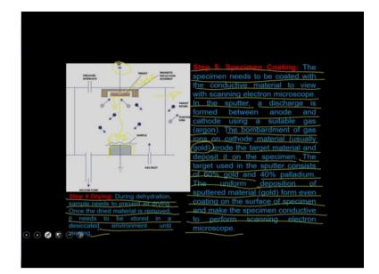
So, after that you have to do a drying step. So in Step 5, you have to do a drying so during dehydration sample needs to prevent air drying. Once the dried sample is removed, it needs to be stored in a desiccated environment, until the viewing. So this means once your sample is been dehydrated you have to do a drying under the vacuum and then you have to keep the sample under the vacuum so that it should not capture the moisture from the atmosphere.
