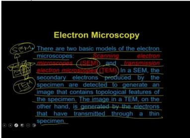
So, there are 2 basic modes of the electron microscopes, one is called as a scanning electron microscope or the SEM and other ones called as that transmission electron microscope or the TEM. So, if you have a sample, you can actually have the 2 things to observe, one how the surface of this particular object and that actually you can do simply by looking at doing with the SEM which is called as the scanning electron microscope.
