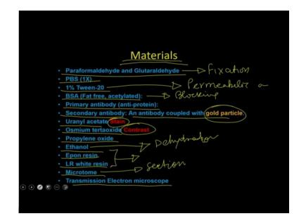
So, these are the material what you require, if you want to do a transmission electron microscope, you require a paraformaldehyde and a glutaraldehyde. So that is you require for fixation of the sample. Then you require the PBS which is generally for the washing, then you require the triton x 100 that is for the permeabilizations, then you require the BSA that is for the blocking.
