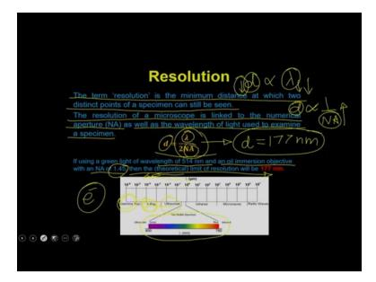
So, the term resolution is the minimum distance at which the 2 distinct point of a specimen can still be seen by the microscope. And by the definition, the resolution of a microscope is linked to the numerical aperture as well as the wavelength of the light used to examine the specimen which means the distance d is directly proportional to the lambda and inversely proportional to the numerical apertures.
