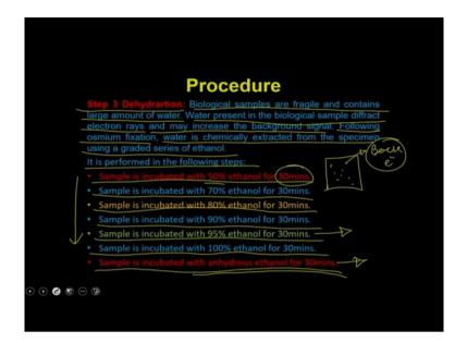
So the water what is present inside a biological sample is actually going to make the sample diffract or scattered the electron beams and that is how it is actually going to make the background more and more pronounced. So to avoid that you have to actually remove the water. So the biological samples are fragile and contains a large amount of water, the water present in the biological sample actually diffracts the electron rays and may increase the background signal.
