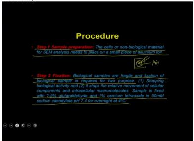
So in the step one, you are going to prepare the samples. So the cell or the non biological material for the SEM analysis need to be placed on to a small piece of aluminum foil. So what you do is you take a small piece of aluminum foil, and then with the help of the pipettes you just deposit your material onto this and then let it be air dry, so that it is actually going to make a thin film.
