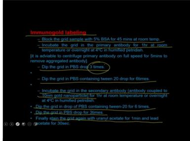
Then you have to do the immunogold labeling. So what you do is you block the grid with the help of the BSA, the incubate the grid in 5 primary antibodies, and then you do a washing to remove the unbound antibodies. So you dip the grid in a PBS for 3 times. And that is actually going to remove the unbound pro antibodies. And then you actually dip the grid in PBS containing tween 20.
