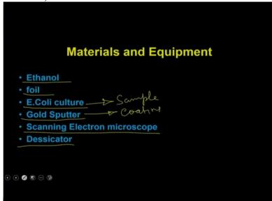
So, how to perform the scanning electron microscopes. So, for to discuss that I have taken an example of the e coli bacteria. So suppose we have to perform the scanning electron microscope of the e coli bacteria and I want to see how the bacteria look like. So material what I required is, I required ethanol, I required the aluminum foil, I required the e coli culture. So, that is the sample what we are going to process.
