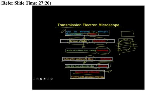
Now, when you do a transmission electron microscope the processing of the sample is little different what you have done for the scanning electron microscope and you have to do additional step because now you want the sample to, electrons to pass through the sample and then actually it is going to give you the image. So, what you have to do is the first step is same that you have to stop the movement of the biological macromolecule which means, you have to do a fixation step.
