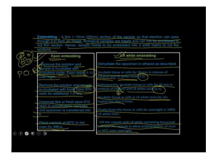
After that, you have to do an embedding. So, a thin 10 nanometer to 100 nanometer section of the sample you have to cut so that the electron can pass through it to form an image. Biological samples are fragile and cannot be processed to cut thin sections. Hence sample need to be embedded in a solid matrix to cut the sections. You have the 2 different types of matrix which you can use, you can use the epon matrix or you can use the LR white embedding.
