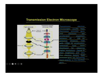
So transmission electron microscope is very simple as it is like a light microscope except that you are using the electronic beam as a source of illumination instead of the light. So I have given you a comparison. So in this case you have a light microscope. So light microscope is using a bulb and that is actually sending the light and then it is being focused by a condenser lens and then it is being illuminated the objects.
