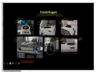
So, when you go into the lab you are going to observe the different types of centrifuges like you have the microfuge, you have the centrifuge like which is going to take up the larger volumes. Then you have the high speed centrifuge and then this is called as the ultra centrifuge which actually can go up to the 1 lakhs G speed or you can have the cold centrifuge or the cell culture centrifuge.
