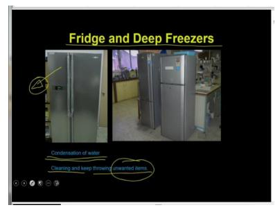
Then we have the fridges and the deep freezers with you know that the fridges and the deep fridges are actually been connected to the compressors. And these compressors actually runs the machines so that there will be a temperature. So, you can have the deep freezers like - 20 and - 80 or you can have the normal fridges. The fridge maintenance are going to be the remain the same as what you do in your home as well.
