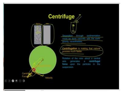
So, you can imagine that sedimentation is nothing but the settling of the material. So, if I suppose take the small mud into a water and mix it and then allow it to settle down the mud will settle down and the water is going to be cleared. So, what this process of settling of the higher particle into the liquid is called as the sedimentation. So, that separation through sedimentation could be done naturally with the earth gravity.
