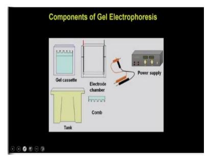
So, these are the components of the vertical gel electrophoresis where you have the gel cassettes, electrode chambers. Then you have the tank where you are going to place this, then you have to have the comb, then you have this electrodes or the power cord. And then you have the power supply unit which is actually going to supply the desirable power between the electrodes. So, these are the electrodes what is being present into the electrode chamber.
