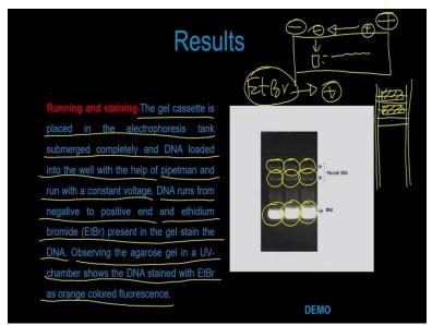
Now the gel cassette is placed in the electrophoresis tank sub submerged completely and the DNA are loaded into the well with the help of a pipetman and run with a constant voltage. So once the gel is prepared then you can just take out the gel from the gel cassette put it into the your your running buffer putting into the electrophoresis chamber and then you connect.
