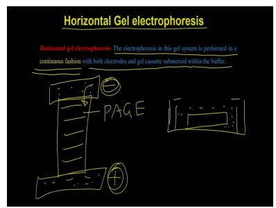
So in the horizontal gel electrophoresis the electrophoresis in this gel system is performed in a continuous passion with the both electrodes and gel cassette are submerged within the buffer. What is mean by the continuous electrophoresis is that the current is not flowing through the gel. Which mean it is actually continuous for example when you are running the vertical gel electrophoresis or if you recall you have the 2 chambers.
