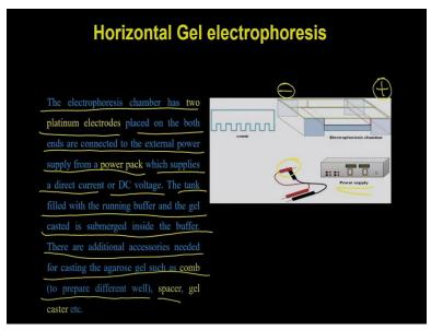
So the electrophoresis chamber has 2 platinum electrodes placed on both the ends and are connected to the external power supply from a power pack which supplies a direct current or the DC voltage. So you have a electrophoresis chamber where you have a negative electrode and the positive electrode on both the side. And then these electrodes are connected to the power cod to the power pack.
