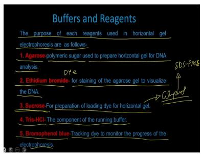
So before discussing about how to run the agarose gel electrophoresis let understand the reagent as well as the instrument what you are required. So for the buffer the purpose of each reagent used in horizontal gel electrophoresis is are as follows. So you require agarose, so agarose is a polymeric sugar which is used to prepare the horizontal gel for the DNA analysis.
