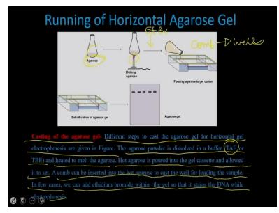
To performing the agarose gel electrophoresis the first you have to cast the gel compare to the acrylamide gel where you are actually going to add the cross linker and then you are going to add the temed and APS to induce the polymerization reactions. Here you are actually not going to do that for casting of the gel. What you are going to do is? You just going to take the agarose. So agarose is the sugar.
