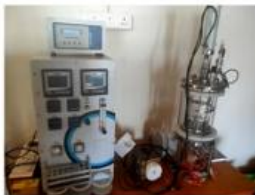
File: A lab-scale biofermenter [Credit: Sarathkumar Ranganathan, CC-BY-SA-4.0, via Wikimedia Commons]
