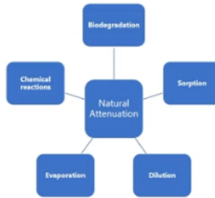
Figure: Processes involved in Natural Attenuation Image generated by author
