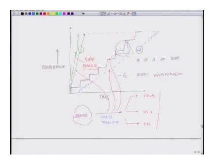
So for example just if you look a slide so depending on for example how you are raising the temperature with respect to time. So on this scale we have time and on this scale you have temperature okay, for depending on how we are increasing it can increase in a stepwise fashion as I was mentioning you over a period of time whatever you will be your temperature you are setting.
