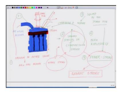
So in terms of the spark ignition engine so it is something like this so it is a more simplistic way I am going to show it purely technical, but do not worry about it okay. So this is a cylinder what is it just drawing okay. And then here you have a spark ignition okay. So this is essentially the spark plug okay, and underneath you have you all have seen inside the scooter the world scooters what you have you will see a spark plug like this and on the side you have something like okay.
