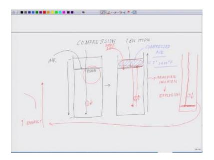
So now talking about the compression ignition this is slightly different so compression ignition works in a different way in compression ignition what happened you have again a cylinder like this in which what you do there is an intake of air simple air okay this is an air intake. And so the air cells, so this is air have filled it up just like the way you saw it in the previous situation then the next step is so once the air is feeling you are moving the system down.
