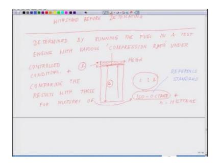
Let me redo it for you, so say for example if this is the piston, so this length which is the length when it fills the whole cylinder vs upon compression when it goes up this length which is I am denoting by small L. So the compression ratio is versus a small L. So high you can compress a mixture without it getting self ignited mix you are much well controlled better feel okay. So it will have a higher octane number.
