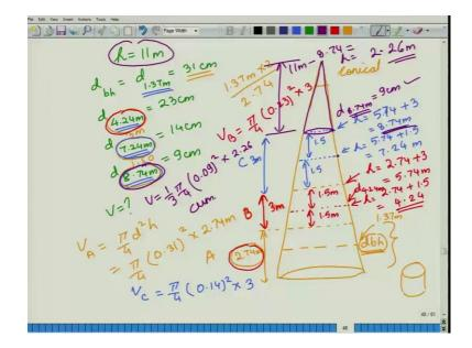
So, let us now try to solve this problem. The total height of the tree h is equal to 11 meters and its diameter at different heights is given the diameter at breast height or the diameter at 1.37 meters is given as 31 centimeters. The diameter at 4.24 meters is given as 23 centimeters, the diameter at 7.24 meters is given as 14 centimeters, the diameter at 8.74 meters is given as 9 centimeters and we need to calculate the volume.
