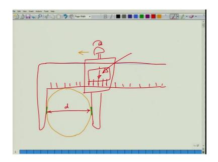
Then we have a moving jaw and a knob here. So, here we will have this scale and this jaw might have a viewing section with a mark and this would tell us what is the reading else.
