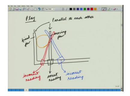
Now what do we mean by play. Play means that when you are taking the readings then both the jaws of the instrument need to be parallel to each other. So, this is the fixed jaw, this is the moving jaw and both these need to be parallel to each other. So, in such a situation, when you take the reading of the tree stem it would be the correct reading; however, in some cases your instrument might be having the play.
