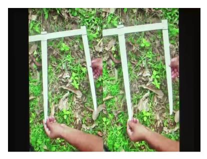
So, in the first situation both the jaws are diverging from each other. In the second situation both the jaws are converging together. So, in both the these situations we will not be getting the correct reading.
