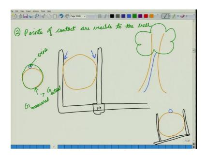
So, if these were your callipers and if you have a tree stem in between; then the user can see this point and this point. So, both the points at which the callipers are in touch with the instrument are visible. So, how does that help? Suppose we had a tree and we had a vine growing on this tree. So, a vine is a climber. So, we had a climber that is growing on this tree.
