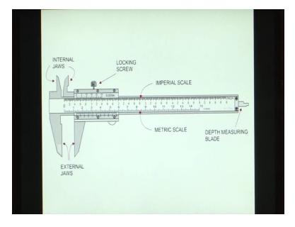
Now, as you can see on this slide this shows a vernier calliper. This is an instrument that most of us have used in our physics labs. A vernier calliper consists of internal jaws external jaws it has a scale that generally has readings in metric as well as imperial scales. It has a depth measuring blade and a locking screw. So, if we drew these callipers we would have, so we have a scale on which we have a fixed jaw.
