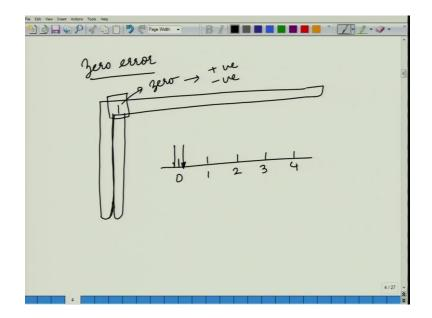
Now, what is what do we mean by 0 error; for instance if we took our instrument and we placed both jaws in touch with each other. So, in this case the reading that we get here should be 0, because both these jaws are touching each other and there is nothing in between these; however, in some cases this reading might not be zero, but might be some positive value or some negative value. What do we mean by a positive value. So,
