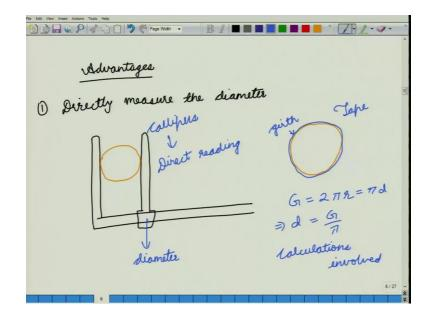
So, what do we have to do to do overcome this error we will need to adjust the instrument and this adjustment might have to be done again and again that being said there are a number of advantages of using callipers advantages.
