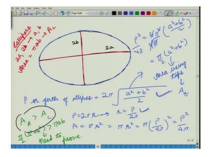
Suppose this is our ellipse. It has the two axis 2a and 2b. So, when we use a tape to measure this ellipse, we are measuring this circumference. So, this is what we measure in the case of a tape. In the case of callipers, we get this reading and we get this reading.
