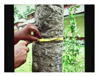
This is an example of an incorrect measurement. So, here we can see that the tape is rolling on itself. So, when it rolls, the diameter of the girth that you would be measuring in this case would be greater than the actual girth of the tree.
