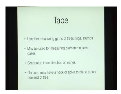
As we know tapes are instruments that are used for measuring girth of trees, logs or stumps. So, when we say girth, we are talking about the circumference. So, when we are using a tape, we will get a circumference.
