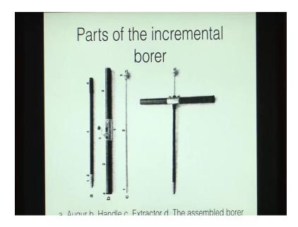
So This slide now tells us the parts of the increment borer. So, it has got 3 parts. Or if you go from left to right it has an auger, a handle and an extractor. And then on the very end we see an assembled borer. So, how does this instrument look like.
