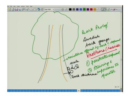
So, to use this instrument you will take the tip. So, it also have a gauge here, and it has a handle here.
