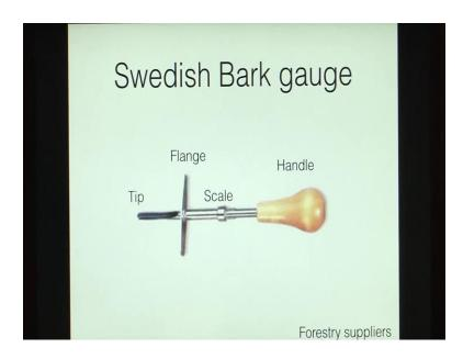
This is the swedish bark gauge. So, this is a measure of indirect measurement. So, as we can see in this image this instrument has a tip now that tip is a sharp tip and it is spent to go inside the bark. It also has a flange it has a scale and a handle. So, how do we use this instrument? So, again considering a tree with a bark.
