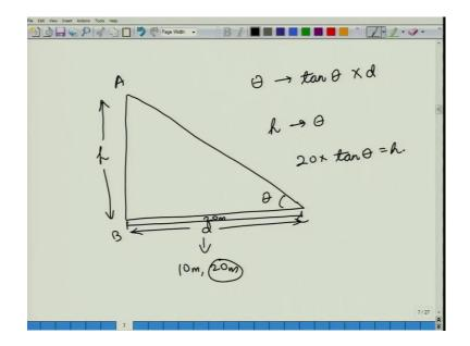
A B C this angle is theta; we take this distance d to be a constant. So, by using the instrument we can take this d to be equal to say 10 meters or say 20 meters depending on this scales as i given in that instrument.
