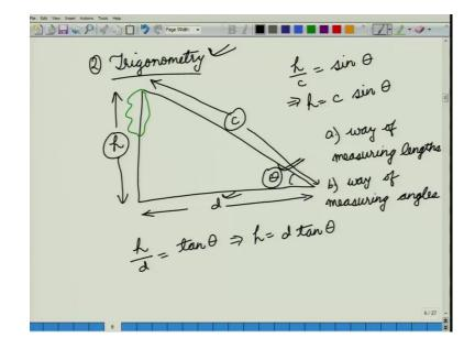
Now trigonometry was dealt with in an earlier class. So, what we do in the case of trigonometry is suppose this is our tree, and we can measure the distance D from the tree to a point of observation and if you can measure this angle theta and we want this height of the tree.
