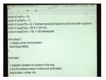
So, we have in the code we have defined are trigger pins. So, because this device is connected to hard you know. So, we have defined it is trigger pins and the echo pins we have also defined a buzzer pin and a beep frequency and beep time. So, when we initialise this code.
