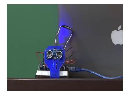
This is an ultrasonic range finder. So, it has got 2 ends. So, when end gives out ultrasonic pulses. They interact with the object in front of it and then they get reflected back to the instrument and the time that is elapse between the emission of a pulse to this pulse coming back to the device is used to get an idea of the distance of the object from the instrument.
