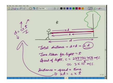
So, this is the point to which you want to take the measurements. And suppose you are standing here with the rangefinder in your hands. So, how would this rangefinder measure the distance? It would give out a ray of light. So, it is a laser light, this light would go interact with the surface of the tree and then get reflected back.
