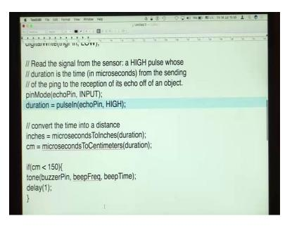
So, it will measure the time during which the echo pin is set to a high. Then it will convert this time into a distance. So, we can measure these distances in inches or in centimetres.
