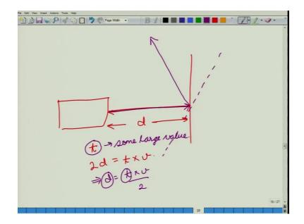
So, our device so, it is giving out a pulse that is going to the object. And this pulse when it returns it takes the time t and then calculates distance as 2 d is equal to t times the velocity.
