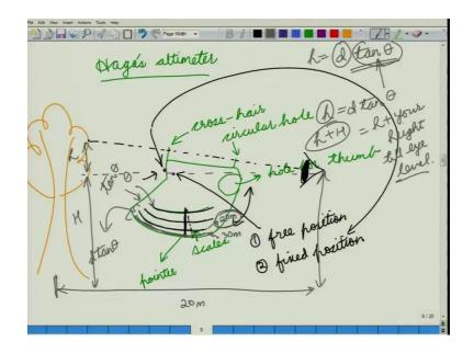
So, how does his equipment function? Now coming back to the on to the slide. So, as you can see this instrument on it is right side it has a circular hole in which you can put your thumb, then on the top you can see 2 ends on the left end and the right end. Now both these ends have to be matched together and the line of site should go to the point where you want to take the measurements. And then downside you can see a number of scales that can be used for measurement.
