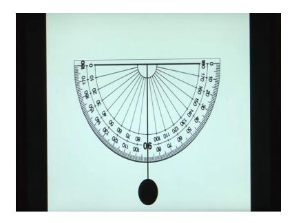
So, what we have done here is we have taken a protractor and right through it is 0 point we have drilled a hole and we have put a string through it. And on that string we can suspend a weight. Now if a weight is suspended then this string is always held vertical. So now, if this protractor is moved to measure any angles it can be used. So, let us now see how it would look in practice.
