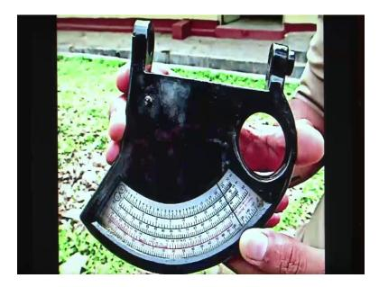
So, this is that instrument it goes by the name of hagas altimeter hagas altimeter.
