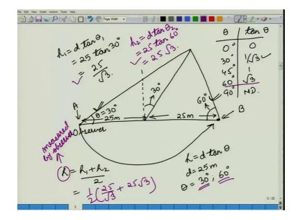
And there is a tree that is leaning away from the observer. So, this is the point of the observer. So, he lies on the ground at a distance of 25 meters from the base of the tree, and he measures the angle to the top. So, he has measured this angle.
