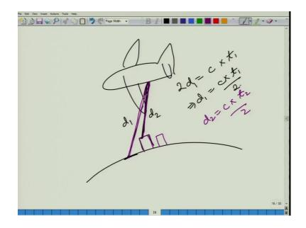
Now, what our aircraft is doing now is that it is flying overhead and then, it is using a laser beam to scan things. So, suppose our ground, suppose we had a building here. So, when the laser beam comes here, it comes and then, it interacts with the surface and then, it is reflected back here it interacts with the ground surface and it is reflected back. So, we can calculate this distance d 1 and calculate the distance d 2 as well.
