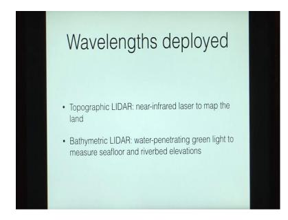
So, we deployed two kinds of wavelength and LIDAR in the case of topographic LIDAR that we use for ground surfaces, we use a near-infrared laser to map the land.
