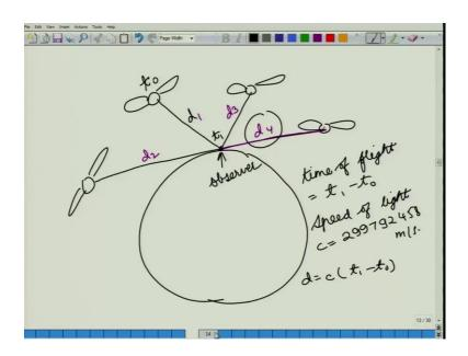
Now, in the case of a differential GPS, we have a constellation of satellites moving above us. So, suppose this is the earth and we have a number of satellites for GPS that are going all around it. Now, if you want to know the position of this particular point, we can calculate its distance from a number of satellites. So, these satellites would be beaming energy from this point of the observer can be calculated by measuring the time difference this signal takes to reach this point.
