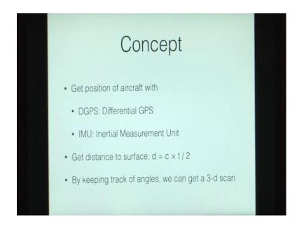
So, what is the concept of using LIDAR and when we are using LIDAR, we need to get the position of the aircraft. Now, the position of the aircraft can be added using two systems. You can use a differential GPS or you can use an inertial measurement use unit.
