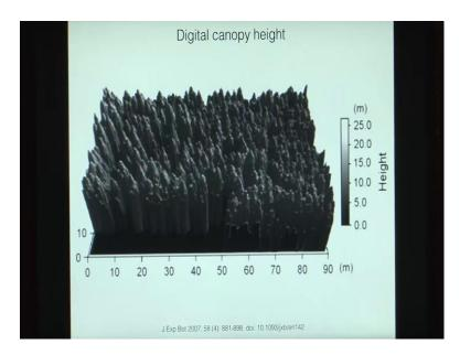
So, in this case we are using all those radiations that are reflecting out from the treetops and then, we are also using this digital elevation measurement to get the elevation of the ground. So, we can get the height of the canopies and we can also use it to get the carbon stocks.
