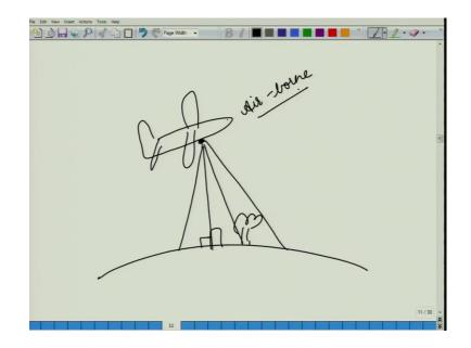
So, when we see an airborne fashion, what we mean is that suppose you have a plane and you can put your LIDAR device here and suppose it is going above the earth, it is getting some buildings maybe a few trees. So, now this laser light would be scanning the whole region in different ways that will come to in this lecture and it can be used in an airborne fashion
