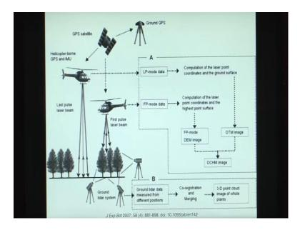
So, this is how scanning would look like. We could go for ground based scanning which would be called a ground LIDAR system. We could put it on in aircrafts, in aeroplane or a helicopter. We could even put it on a satellite or you could put it anywhere essentially, but you need to know your position, you need to know all the angles and you need to calculate the time of flight of the laser beams.
