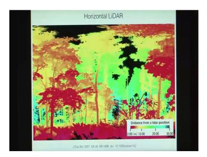
So, in the case of this horizontal LIDAR, these different colours are showing the distances from the LIDAR. So, for instance this tree is close by as compared to this tree. So, here we have put our LIDAR out there on the ground and that is scanning the whole forest region and once it has scanned the whole region, it will give you this picture of the forest.
