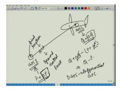
So, we would have GPS1 that is kept at a fixed location also known as GCP that stands for Ground Control Point.
