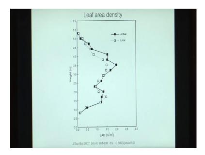
Now, this 3D picture can be used to to compute the leaf area density. So, in this graph we are seeing the leaf area density as computed from LIDAR and as computed physically from a tree. So, as we can see there is a very good correlation between both of these. Now, if we have this 3D picture of a tree, we can also use it to compute the canopy height.
