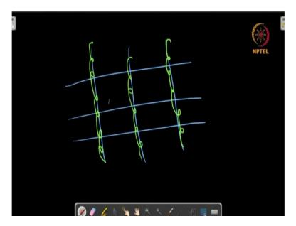
And typically, the support is provided in the form of a pattern that looks like this, so you can have this structure and if you give it to the climber then the climbers will climb like this, so this is a trellis pattern. So, in the trailer pattern you can have vertical rods or you
