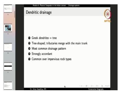
What kinds of drainages do rivers make. The most common drainage is the Dendritic drainage, the term comes from the Greek word dendrites which means a tree, so this is a tree shaped drainage where tributaries merge with the main trunk.
