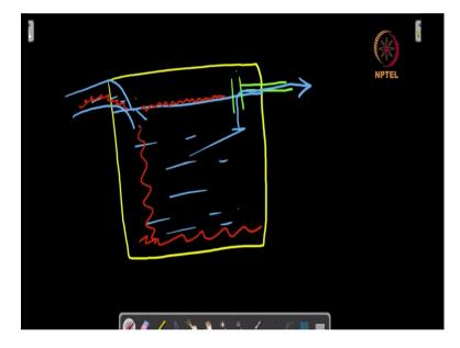
So, the way a septic tank works is that you have a large size tank which is covered and the sewage moves into this tank through a pipe and there is a layer of water that is maintained in the septic tank. So, in this case all the sewage will either move down to the bottom of the septic tank or it will stay here on the top as a sludge.
