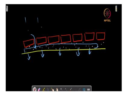
Now in the case of paving blocks what happens is that above the ground surface so if we went for concreting it would be a completely impervious layer of concrete that would be poured, but in the case of paving blocks a layer of sand is added to the top of soil and above this layer we put blocks which are made out of burnt clay.
