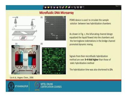
So, here that microfluidic DNA microarray; basic principle is that you have a microarray chip where that microarrays are spotted. And your samples would be passed through that chip with a shortened speed and with a some additional some attributes like say oscillating flaps and etcetera by which that surface concentration of that DNA molecules which will be probed, means which will be accessed there will be concentration will be increased.
