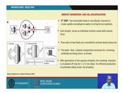
So, this is the in details of that your droplet generation and cell encapsulation process. This is 2 and 3 these are the aqueous compartment which one compartment containing that your mixture of beads and that fluorescence antibody, then another compartment containings that all the hybridoma cells.
