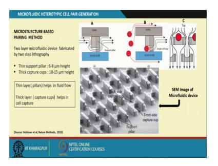
This is very beautiful structures means designing with respect of design and that flow we are of that cells in that microfluidic chip. So, here principle is that you have 2 layer microfluidic device fabricated by 2 step lithography; this is your support pillar and this is a capture cup.
